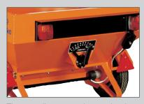
The spreading amount is set using the handle, which controls the spring base adjustment.
